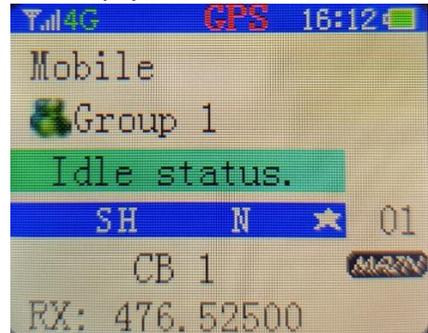
The TA-680 has a simultaneous dual screen of both modes; Network and UHF. The upper half is the Network mode with the green status bar. The lower half is the UHF mode with the blue status bar. The **MAIN** icon shows the current active selected mode.
